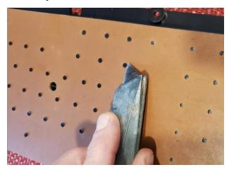
Go slowly when separating the hard backing plate so as to not break any of the plastic pegs. These are essential to hold everything together!
