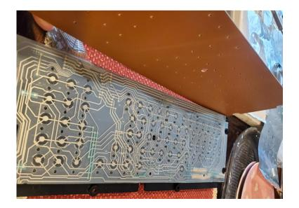
Next, remove the remainder of the membrane assembly, which consists of two layers of Mylar with circuit traces running all over, and a clear blank Mylar sheet that is exactly like the first sheet you removed. The difference is that this sheet lies between the latter two circuit sheets.
