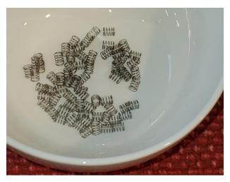
At this point, with all the tiny springs removed and safely stored, the large plastic keyboard structure is now ready for a good soap scrubbing. Used a light brush (old toothbrush) with dish washing liquid to clean all of the aforementioned junk out, and then give it a good rinse and set it out to dry.
