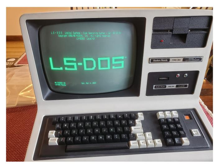
After purchasing my TRS-80 Model 4GA and working to get out up and running, I quickly discovered that several important keyboard keys weren't functioning correctly. The shift keys were displaying the I and H characters (see picture) respectively and the B, H, I, J, K, L, and N keys were all behaving erratically. Since both shift keys were not functioning correctly there weren't many commands I could carry out.
