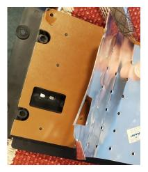
Use a box cutter knife to break off <u>only the tips</u> of each plastic peg (melted fasteners), and then slowly work to remove the hard "Formica-like" (e.g., circuit board material) backing plate.
