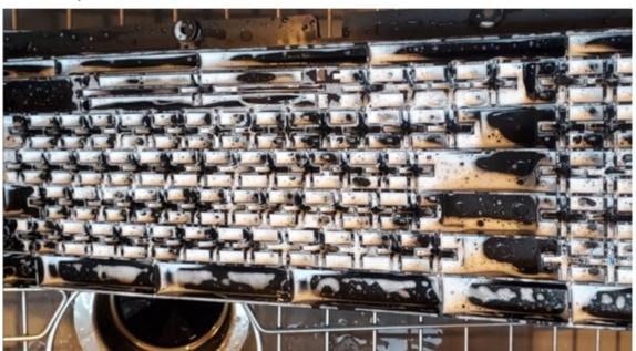
Once the keyboard structure is dry, it is time to put everything back together. Carefully replace each and every "under key" tiny spring.
